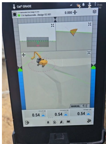
Cat GRADE display showing 0.54m fill readings, consistent across all three bucket positions — confirming stable correction lock
